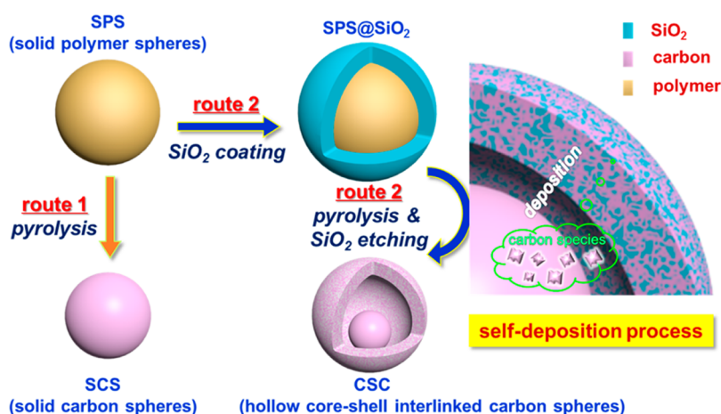
Figure 1. Schematic illustration of the synthesis of the hollow core–shell interlinked carbon spheres.
